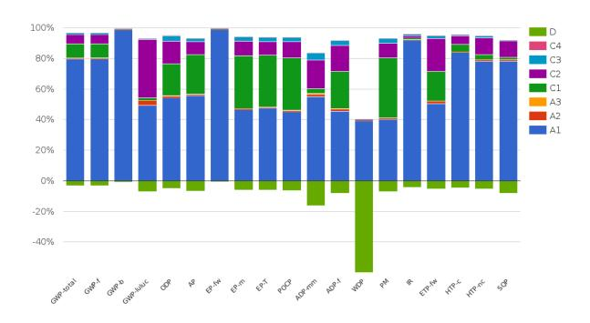
The figure illustrates the impact categories for 1 m<sup>2</sup> of concrete paving stones.
